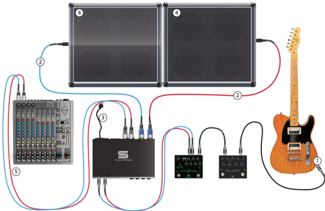
Use high quality **speaker cable(s) [2]** to connect your PowerStage 700's **Speaker Output Jack(s)** to the input of a **4 - 16 ohm cabinet [4]** or cabinets. PowerStage 700 uses Neutrik combi-jacks for compatibility with both speakON and quarter-inch speaker cables. Using the supplied **power cable [3]**, connect the PowerStage 700 to a power outlet.
